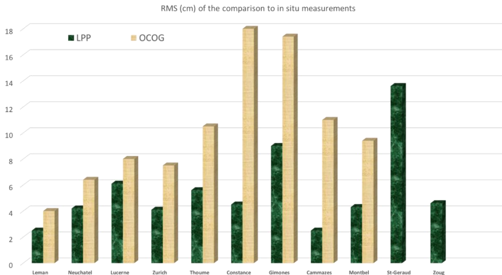
Figure 2: summary of RMS differences between in-situ measurements and WSH calculated using LPP and OCOG retracker, for lakes in Occitanie and Switzerland.
