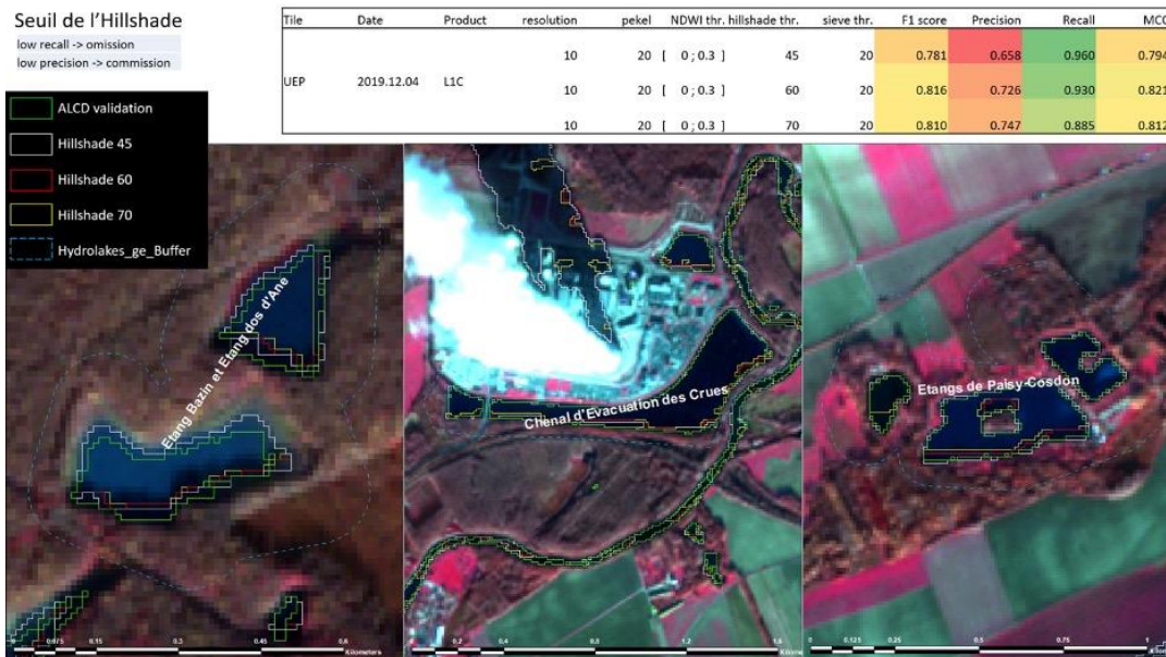
Figure 14: Evaluation of the hillshade values of water recognition and impact on score's values (ALCD reference database from Pena Luque et al (2021).
