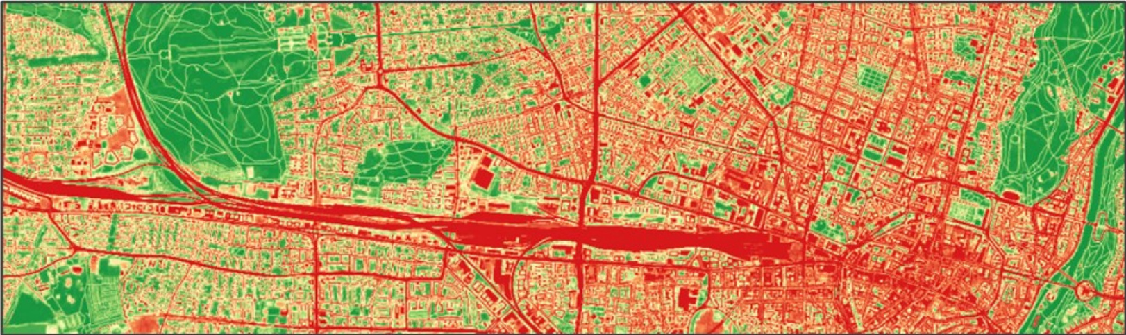
Mapping of imperviousness/greenness [10m] within the built-up area based on analysis of multi-seasonal Sentinel-2 imagery
