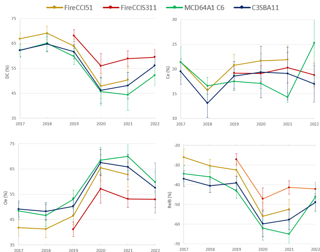
Figure 34. Accuracy metrics (DC=dice coefficient, Ce=commission error, Oe=omission error, relB=relative bias) for each calendar year for the four global products analysed FireCCI51 (yellow), FireCCIS311 (red), C3SBA11 (blue) and MCD64A1 C6 (green).
