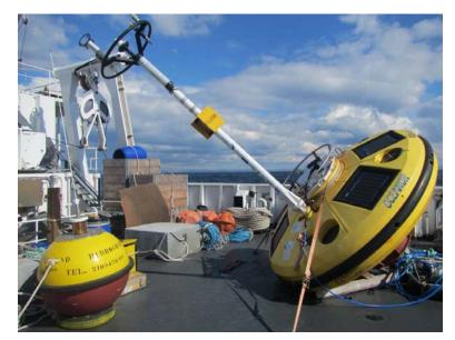
Figure 6-16. Oceanographic Datawell Waverider (left) and Meteo-oceanographic Oceanor Wavescan (right) buoys (photo © Instituto Hidrográfico).
