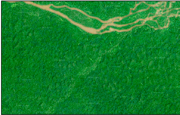
Figure 3-16: Example of topography-induced modulation of AGB estimates (top) and corresponding optical image from Google Earth to be considered as reference for the landscape (bottom). Uncompensated topography caused a variation of up to 200 \text{ M g ha}^{-1} between slopes facing the radar (light green areas) and slopes looking away from the radar (dark green areas).
