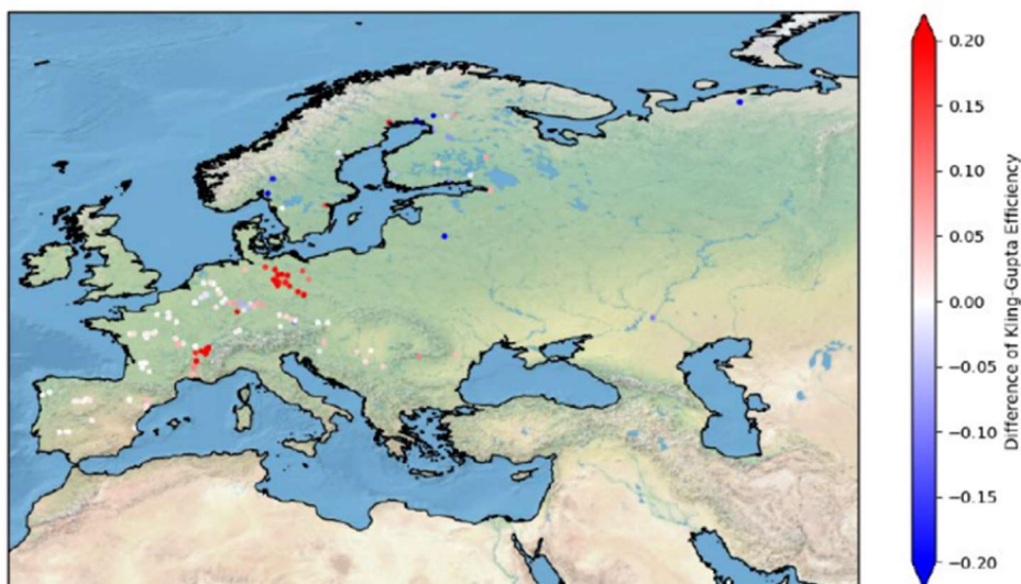
Figure 3.2.3: Impact of assimilating SWE on the Kling-Gupta Efficiency score of river discharge over Europe.
