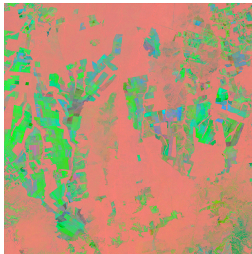
Figure 3-37: RGB composite of the time series parameters a_0, a_1 , and b_1 estimated from an annual stack of VH backscatter imagery acquired in 2018 over an area in Mato Grosso, Brazil.
