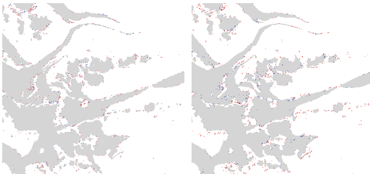
Fig. 3.7: Left: Three glacier maps combined resulting from three threshold values: 1.8 (all colours), 1.9: (grey and blue), 2.0 (grey). Right: Effect of a 3 \times 3 median filter: red pixels are removed and blue pixels are added (shown here for the map with the threshold 1.9).
