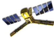
SMOS L-band (ESA) Interferometric Radiometer Spatial res~43 km (30-80 kms) Swath~1500 km Revisit-time~2-3 days Incidence 0°-60° Full polarization Launched Nov 2009
