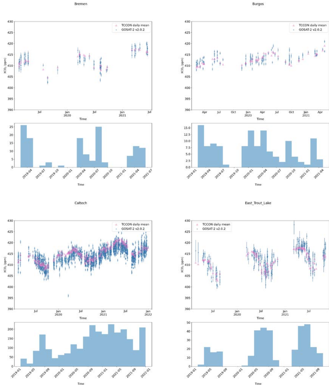
Figure 5-3-1: Comparison of land single soundings of XCO 2 from the full physics retrieval (blue circles) with co-located TCCON (pink triangles) measurements at all TCCON sites for the period Feb 1919 to Dec 2021. Histograms are also given for each station indicating the number of GOSAT-2 retrievals present throughout the time series.
