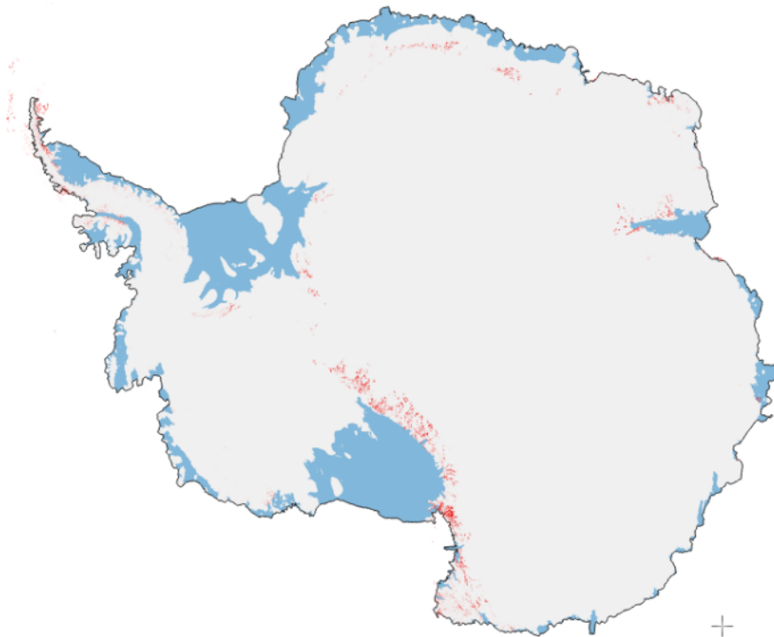
Figure 3-2: Map of Antarctica showing in blue floating ice shelves and in red the rock outcrop shapefile used for the stable terrain test (Burton-Johnson et al., 2016).
